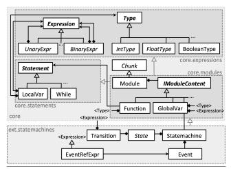
**Figure 8.** Class diagram that illustrates some of the core structures and dependencies in mbeddr. Italics text denotes abstract concepts, bold text represents important extension points, names in angle brackets act as proxies for the named concept to avoid even more lines. Details about the design are explained in the running text.
