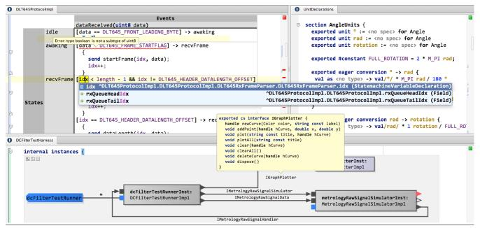
**Figure 1.** The screenshot shows various parts of the mbeddr languages: a part of a protocol parser state machine (top left), unit declarations (top right) and component wiring for a test case (bottom). It also illustrates how mbeddr provides IDE support for C and its extensions, including syntax highlighting, code completion, error markup, refactorings, quick fixes and tooltips. The screenshot also showcases the support for mixed notations (text, tables, diagrams).
