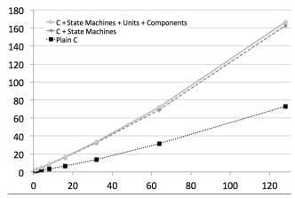
**Figure 17.** Generation time (in seconds) for a single, synthesized model depending on the number of roots with 1,000 nodes each. The model with 128 roots corresponded to 68,400 LoC of generated C code (for Plain C), 202,000 LoC (C + State Machines) and 198,000 LoC (C + State Machines) + Units + Components). The data was measured on a Macbook Pro, 2.7 GHz Core i7, 8GB RAM.
