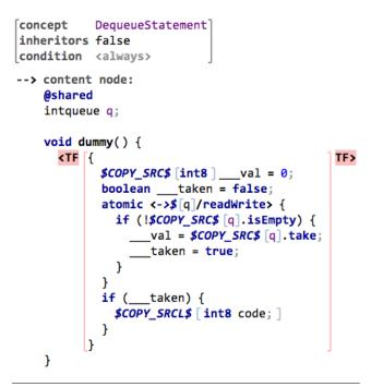
**Figure 4.** The generator templates used for translating the DequeueStatement. The dummy function acts as scaffolding for the template fragment; the details are explained in the text.
